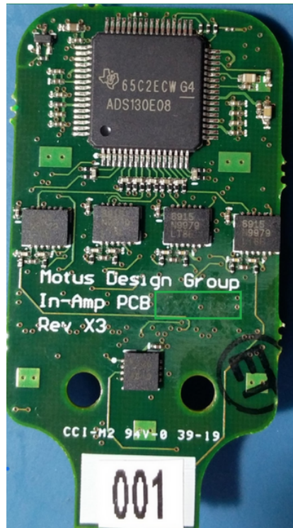
Custom digitally controlled instrumentation amplifier PCB
